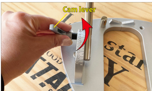
⑤ Tilt the Cam lever backward to loosen it. Adjust the angle and tighten the left and right Cam levers.
