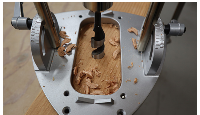
Centred holes in squared timber
