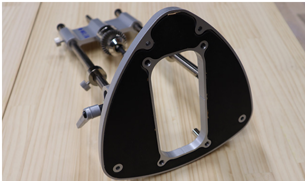
The bottom of the base has a rubber sheet to prevent slipping.
